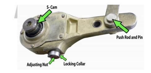
**Explain Examiner**: Tight brakes all the way same direction S-Cam moving then loose 1/3 and check push-rod travel  $\frac{1}{2}$  to  $\frac{3}{4}$  inch. Make sure lock is out.
